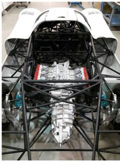
Next steps for the engine were to design the exhaust systems, and BTB were fantastic in working with us to make sure my designs were feasible to manufacture. Twin CATS, and twin vertical silencers so the rear view would look like a 917, no unsightly silencers slung across the rear. We choose Jenvey throttle bodies, latest Bosch injectors, and a DTA ECU to ensure that we would meet the IVA test emission requirements.
