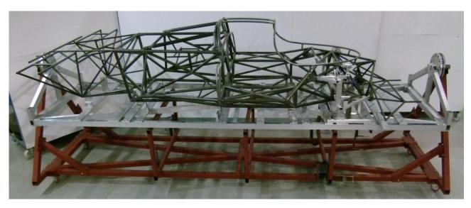
The jigs and chassis were built by ARK Engineering at their Basildon facility to my designs from approx. 217 T45 steel 5 axis laser-cut tubes rather than the original aluminium to meet modern safety regulations if we ever go for FIA Continuation approval.. But otherwise chassis is very accurate (within 5 to 10mm) of the original apart from the alterations for the 964 engine and G50 transmission.
